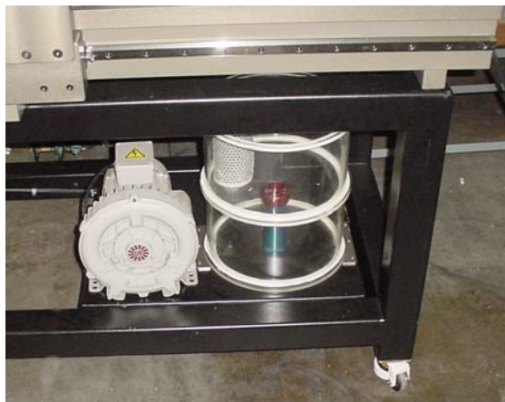
High Capacity Chip Collection & Lubrication System. Heavy duty engraver stand with locking casters. Stand contains all electrical and controller components.
